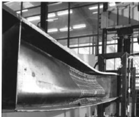
Figure 2. Vertical web buckling.
